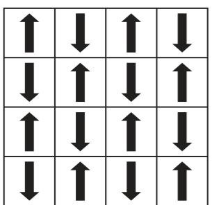
**OPPOSITE DIRECTION** – Tiles should be placed one beside the other, but in the opposite direction, so that the arrows on the backside of every next tile are under the angle of 180° compared to arrows on the previous tile.
