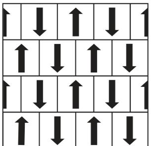
**THE TILES IN THE HORIZONTAL ROWS ARE PLACED ONE BESIDE THE OTHER**, so that all arrows in the back of tiles have the opposite direction (every next tile is placed under the angle of 180° comparing to the previous). Every next row is set on the same way but it begins in the half of the tile from previous row.
